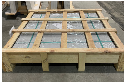
Packaging in a crate for large-format flooring
