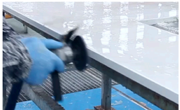
1.5.1. Smooth finish to dissipate stresses.
