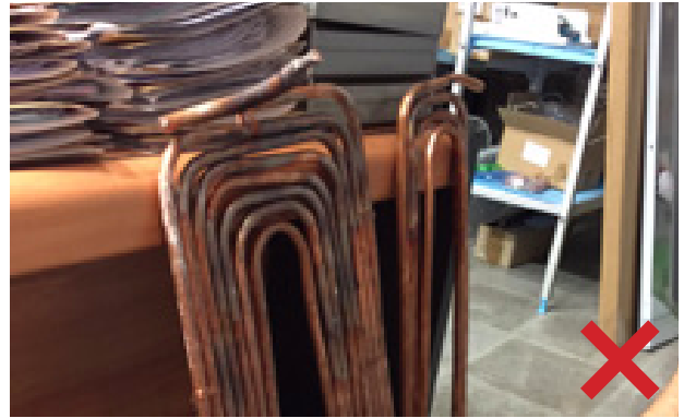
5.4.1. A higher copper tube density does not guarantee a good result. The key is to flatten the tube to gain contact surface, because the cold has a tendency to go down to the frame instead of going up to the countertop.
