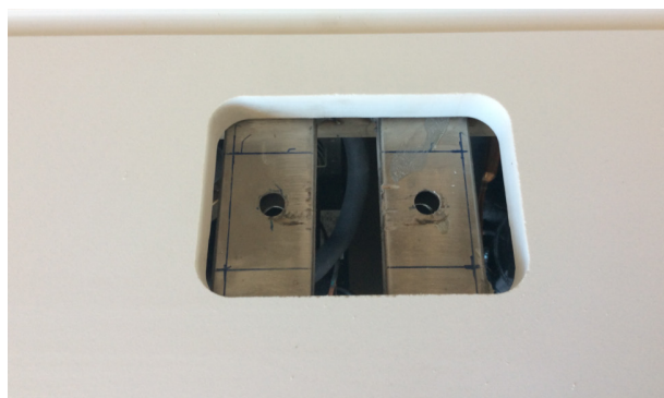
4.1.4. The screen posts are directly fixed to the chassis.
