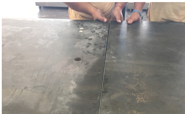
4.1.2. Drill hole away from joints (another piece in large plates). Do not drill in joints.
