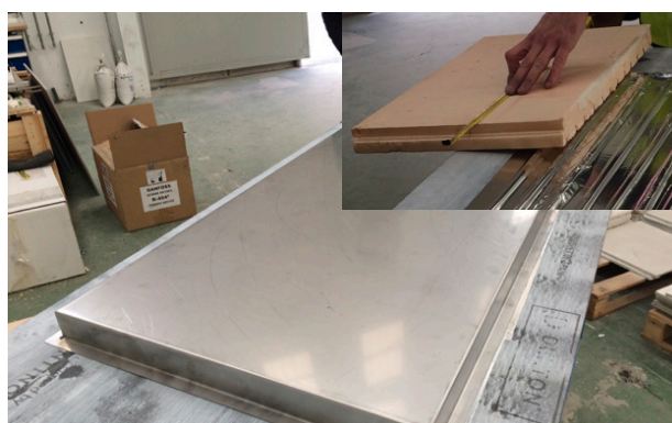
5.1.4. Sufficient insulation underneath to prevent cold losses and condensation on the chassis.
