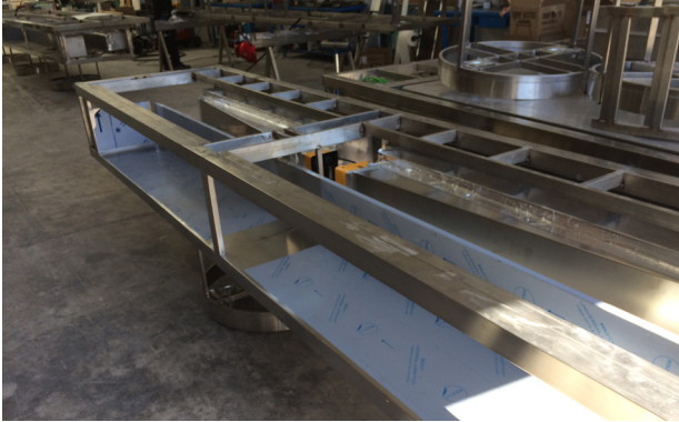
2.2.1. Large spans with fewer transverse frames can be saved when horizontal levels (upper and lower) are very rigid and there is no risk of long-term arrows greater than 1 mm.
