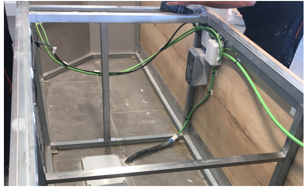
2.2.3. Example of a transverse frame that lowers its elevation to be distant from the integrated cold or hot plates.
