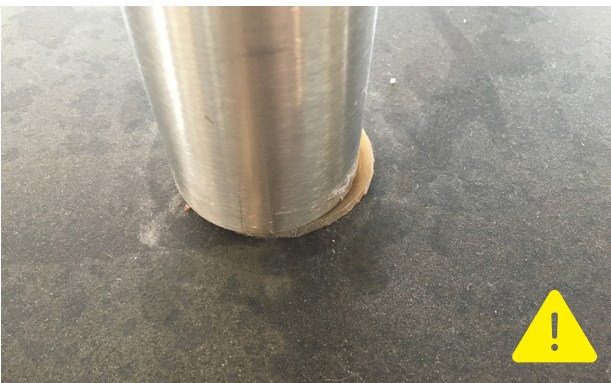
4.2.3. This type of support of the post can cause overstressing on the worktop.
