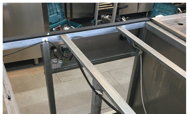
3.1.6. Placing on the entire support surface of the upper frame level.
