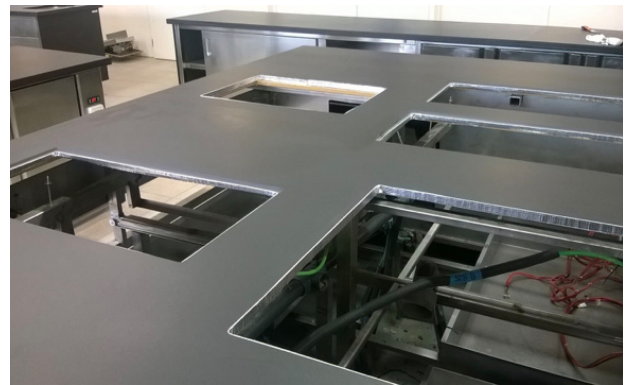
1.2.1. Distances between cut-outs and the edges of the countertop.
