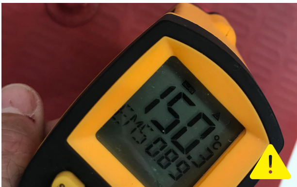
6.5.1. The etched foil must not emit heat above 120 °C.
