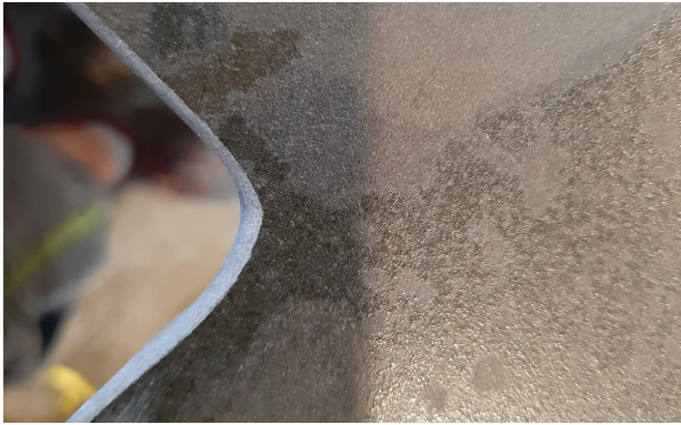
1.3.1. Inner radius with rounded finish.
