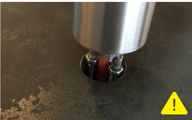
4.2.2. Ideally the post should also pass through itself until it reaches the chassis.
