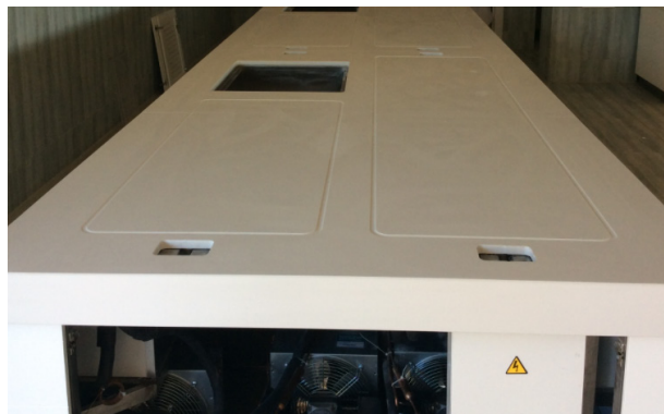
4.1.3. Through holes for supporting the posts on the chassis.
