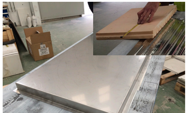
6.2.4. Sufficient insulation underneath to prevent heat loss and chassis overheating.
