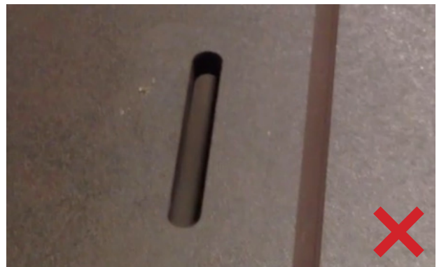
4.3.2. This groove does not meet the specified minimum width and does not allow the post to pass through.
