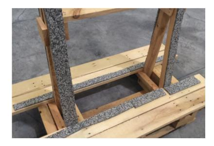
SAfter loading every piece on the pertinent trestle, secure the load with hoops, preventing direct contact between the hoops and the edges of each piece.
