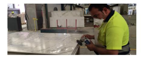
Before cutting each slab, it is important to mark each cut point and identify each piece with the pertinent references. Besides, it is recommended to gather the already cut adjoining pieces together, in order to check the perfect vein matching. Pay special attention to the main or more characteristic veins. Once the vein matching is being checked, mark the final cut points and proceed cutting. Repetir este proceso para el corte de todas las tablas.
