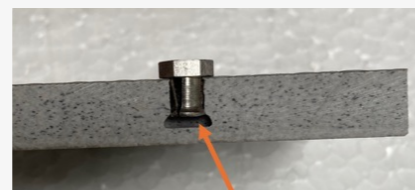
Water Penetration in hole
