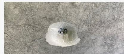
Pictures with examples of chippings produced by water penetration into the drills, combined with freezing temperatures, causing the product breakage.
