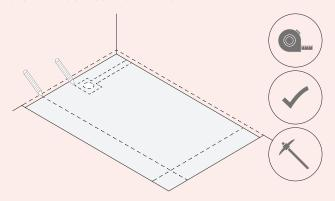
b. Once there is enough space for the installation of the drainage system, make the relevant connections to the drain pipe in the bathroom, ensuring a slope of at least 2%.
