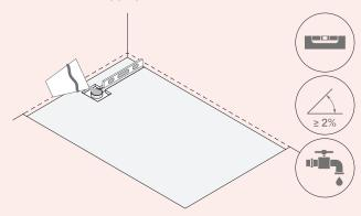
c. Make the necessary slopes towards the drainage system with mortar, using a trowel or metal screed to smooth it, and ensuring a minimum slope of 2%. Allow it to dry for at least 24 hours.
