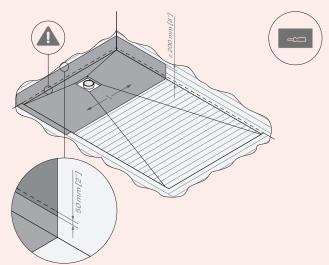
g. Prepare and spread the adhesive uniformly, both over the entire surface (ensuring that the membrane does not tear) and on the back side of the tiles, using a notched trowel.
