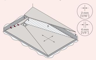
i. When filling the joints between tiles, choose the grout suitable for wet areas and the desired color and apply it as per the manufacturer's instructions. After a few minutes, wipe off any residue with a damp cloth and let it dry for at least 24 hours.
