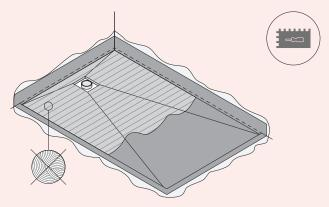
h. Install the Dekton® Grip/Grip+ tiles according to the cut for each of the slopes executed, leaving a minimum recommended joint of 2 mm [1/16"] between pieces and 4 mm [1/8"] along the perimeter against the walls. We recommend the use of spacers to maintain this joint width and leveling tools for large format tiles.
