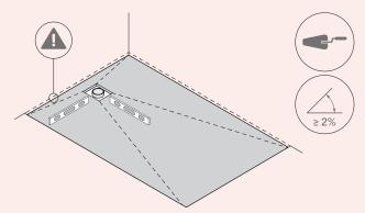
d. Place the waterproofing membrane over the substrate to ensure that it completely covers the shower area and lift it onto the adjacent walls by at least 200 mm [8"]. Once the dimensions have been checked, remove the membrane.
