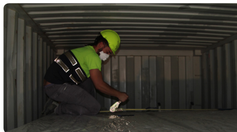
Tightening with the ratchet system
