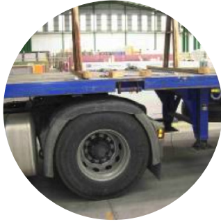
Placing of front rack (on the axle).
