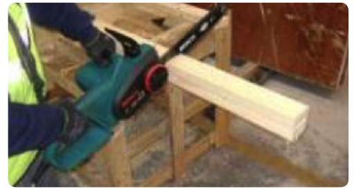
Step 4: 4 pieces of wood are cut to size to fasten the planks to each other.
