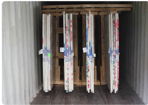
The loads must be equidistant from each other.
