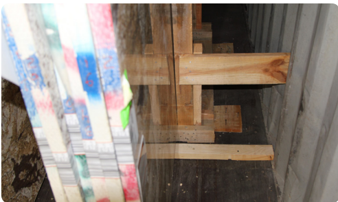
Detail of the lateral anchoring in the second row of the load.
