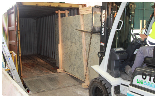
To protect the edge of the bay, the pallet base is raised a few centimetres.
