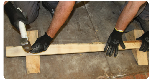
Creating the chock inside the trailer.
