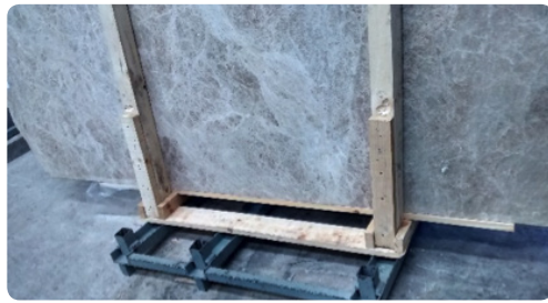
Step 1: Placing the planks at both sides.
