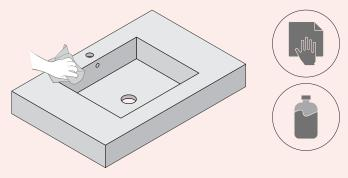
f. Seal the joint between the washbasin and the wall with anti-mold silicone. Smooth the silicone bead and let it dry for at least 24 hours.
