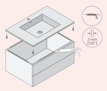
b. Immediately afterwards, place the washbasin on top of the bathroom cabinet, making sure that the washbasin is centered and leveled.
