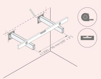
$\rightarrow$  If the basin has a double sink, it will be necessary to place a third intermediate support bar at an equidistant position.
