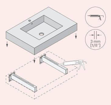
d. Immediately afterwards, place the washbasin on top of the support bars, making sure that the washbasin is centered and leveled.
