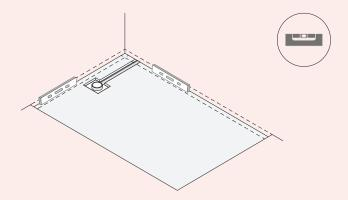
d. Present the shower tray in its definitive position, connect the drain valve and verify the correct slope of the support, before the final gluing.
