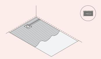
g. Then place the shower tray, leaving a minimum open joint recommended of 3 mm [1/8"] in its perimeter, and press on its entire surface.
