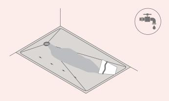
j. Once the vertical cladding and grouting have been done and it is dry, proceed with sealing the perimeter of the shower tray with anti-mold silicone. Wait at least 24 hours for the adhesive to dry and cure completely and clean up any remaining residue.
