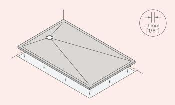
h. Install the drain valve according to the instructions supplied. It is important to do it manually (do not to use electric screwdrivers).
