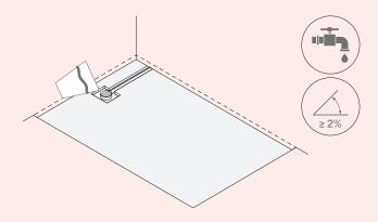
**NOTE**: It is recommended to plug the drain pipe during installation in order to prevent construction debris from falling.
