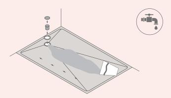
e. Once the initial test is done, disassemble the valve and remove the shower tray to proceed with installation.
