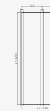
V1. Max. Design wind load: 3.5 kN/m²
