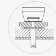
DKR. Riveting (thickness = 4 and 8 mm)
