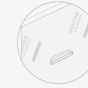
DKB. Intermittent groove on the reverse CR5 (thickness = 8 and 12 mm)
